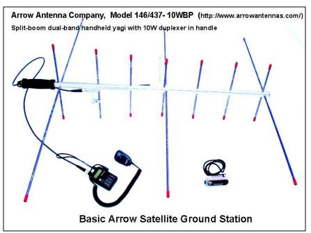
gain on the 2m uplink and about 10 dB gain for the 440 MHz downlink. With this system, I average about 2-4 contacts per pass (with none on some passes).
