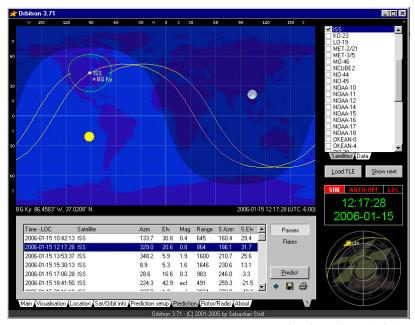
amateur radio satellites, go to <u>http://www.amsat.org/amsat-new/tools/keps.php</u> and select the NASA two-line elements (TLE). Highlight just the data portion of the display, copy, and then paste into a text editor and save the file. It can be loaded into Orbitron to facilitate currently accurate orbital calculations. The data are updated about once per month.
